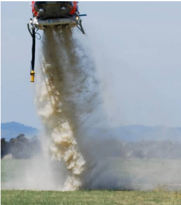
Image shows 1400 litre mixed polymer drop under the influence of a 16 knot partial cross wind.
