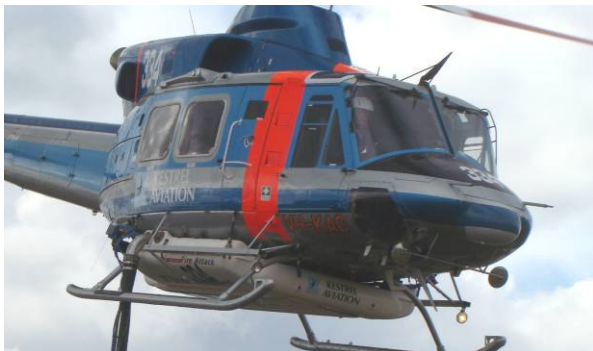
The Bell B412, HTK 334 fitted with the 1400 litres Simplex 304 belly tank.
