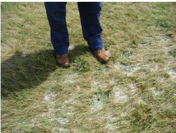
Image shows the distribution of the mixed polymer product within a drop footprint.
