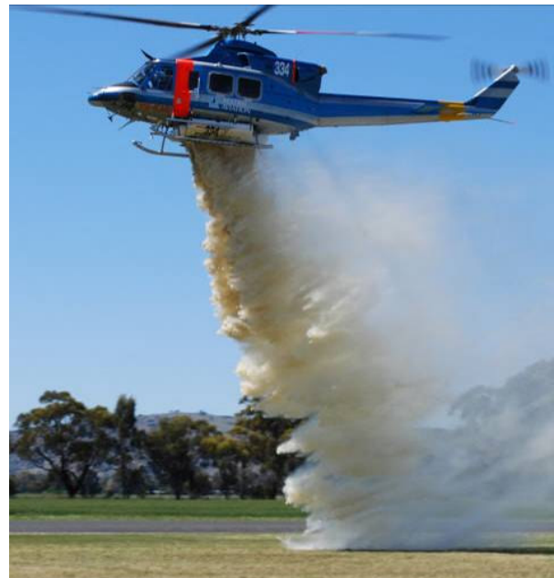
Drop 1 27 Oct 2001, image #2, HTK 334 releases 1400 litres of water and mixed polymer at 0.6% concentration.
