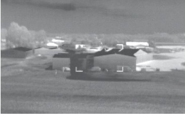
Extracted 90° horizontal infra-red image of 1400 litre mixed polymer drop.
