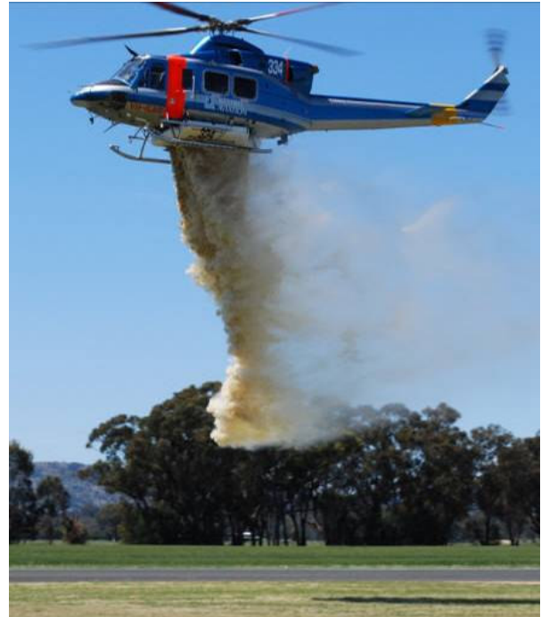
Drop 1 27 Oct 2001, image #1, HTK 334 releases 1400 litres of water and mixed polymer at 0.6% concentration.
